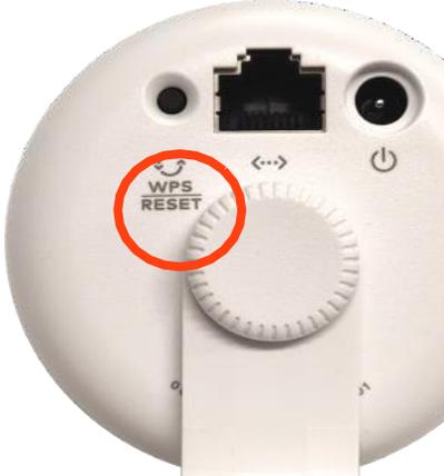
A photograph of the back of a white indoor camera. The camera has a circular shape with a lens on the left and a power button on the right. In the center, there is a circular button with a circular arrow icon and the text 'WPS RESET' below it. This button is circled in red. Above the button is a small Ethernet port and a power button. Below the button is a power button. |
